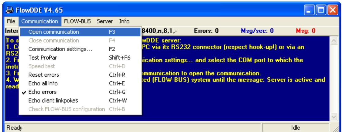
Once the DDE server is active, open the FlowDDE Test Form via the menu (as shown below) or by pressing <F6>.
