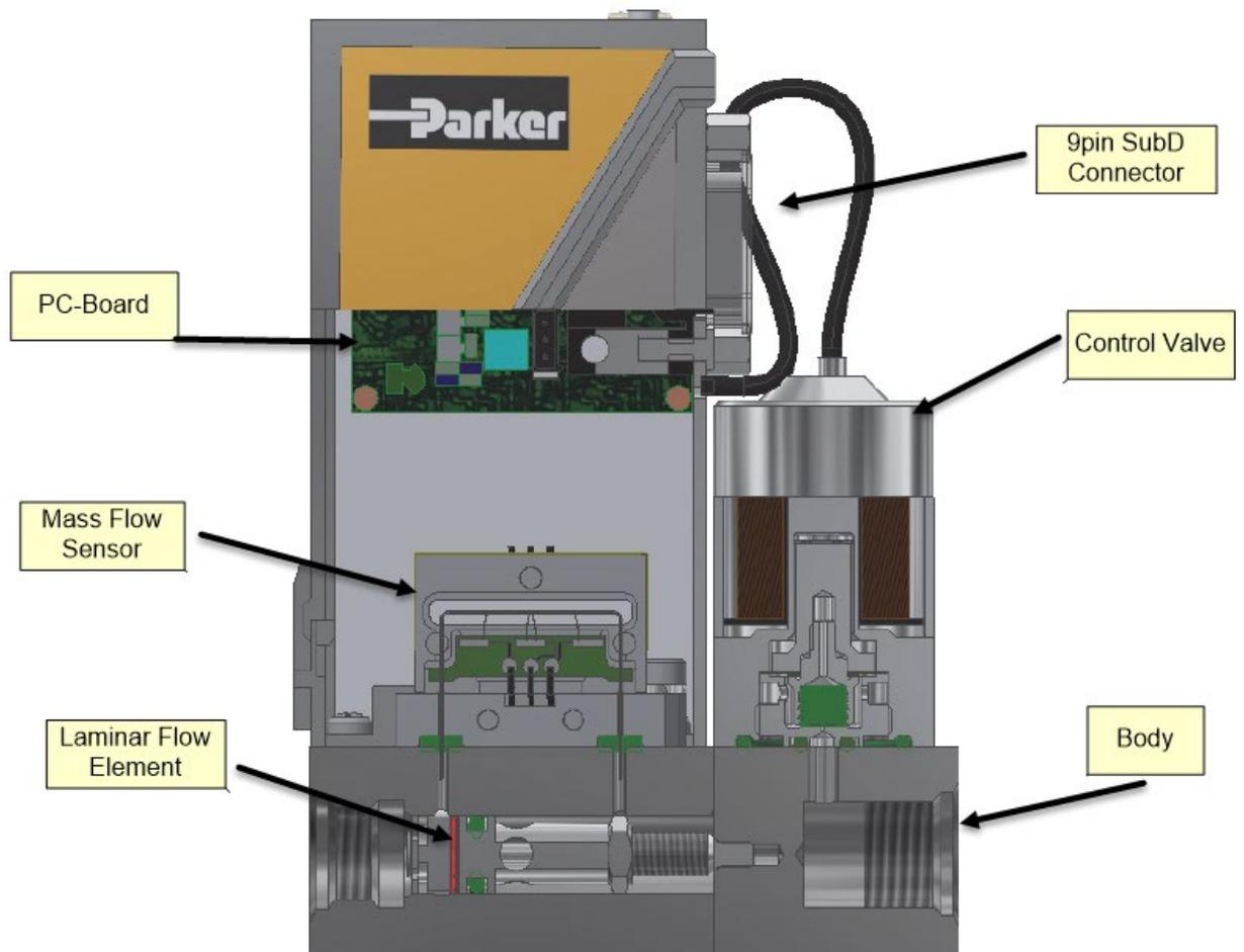
There is one model, 601XF, for flow rates from 40 ml/min to 20 l/min. For simplicity, the standard X-Flow™ configuration is optimized to provide the best repeatable flow measurement possible.
